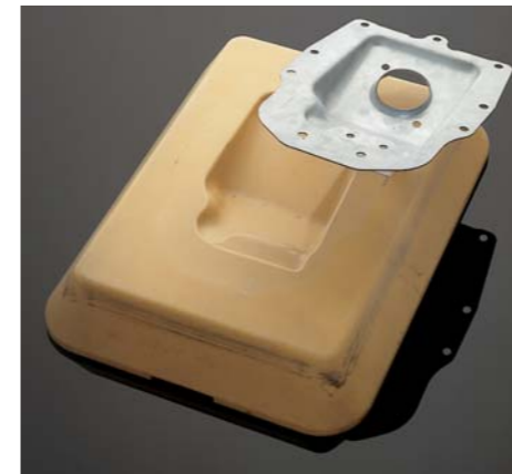
Pressing tool with a 2 mm steel sheet of obomodulan® 1200
