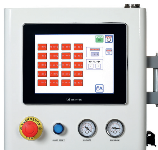
Heaters screen with 20 independent zones
