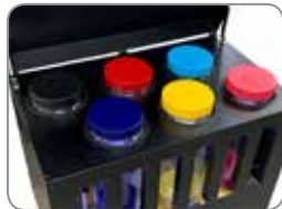
5kg/color continuous ink supply system Designed to be refilled with inks while printing. The level of ink is easy to check visually or by sensor. Is provided with a double filtering system able to protect the printer against any intrusive or harmful substances.
