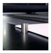
**Registration pins** ensure (up to 1 mm) accurate board alignment, which is particularly relevant for recto-verso printing. Agfa's Asanti software automatically selects a pin set configuration depending on the size of the media.
