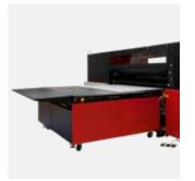
The automatic board feeder (ABF) handles **up to 4 boards** side by side with a maximum length of 1.85 m. Bypass is possible for longer boards (up to 4 m).
