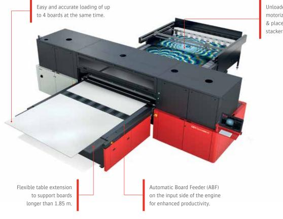
Unloader unit consisting of a motorized conveyor table, pick & place system and scissor stacker for up to 4 stacks.
