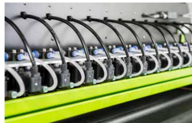
• You can individually choose nozzles and set the dimensions of the area you want to pretreat. A laser system will automatically detect the correct spraying area on the garment.
