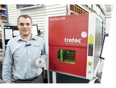
"We use the SpeedMarker 700 to mark the brand and logo on our motors, along with all its specifications and certifications. The system is fully integrated with our ERP, once we scan the work order all the info is automatically pulled. Trotec offers impeccable support especially in the early stages of programming and calibration. The SpeedMarker 700 offers the highest quality of marking on stainless steel and mild steel units. "
