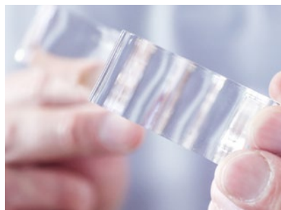
Flame-polished result. Cut up to 40mm acrylic.
